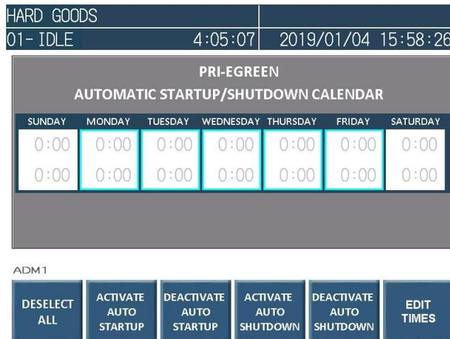
**Figure 6.0-47 AUTO ON/OFF Configuration Buttons**
