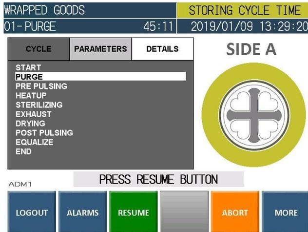
**Figure 9.0-4 HOME Screen With Acknowledged Alarm**
