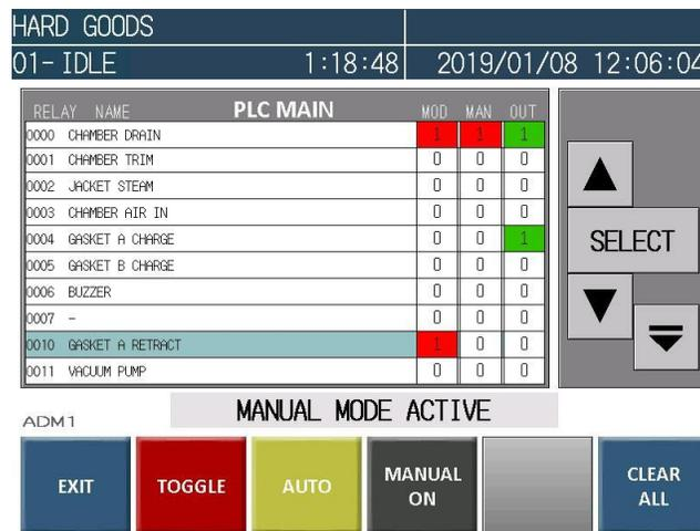
**Figure 6.0-19 DIGITAL OUTPUTS TOGGLE Button**
