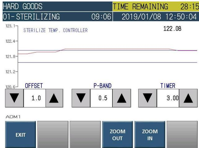
Figure 6.0-36 OFFSET, P-BAND and TIMER Screen
