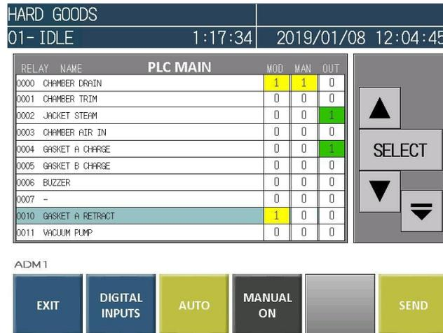
**Figure 6.0-18 DIGITAL OUTPUTS SEND Button**
